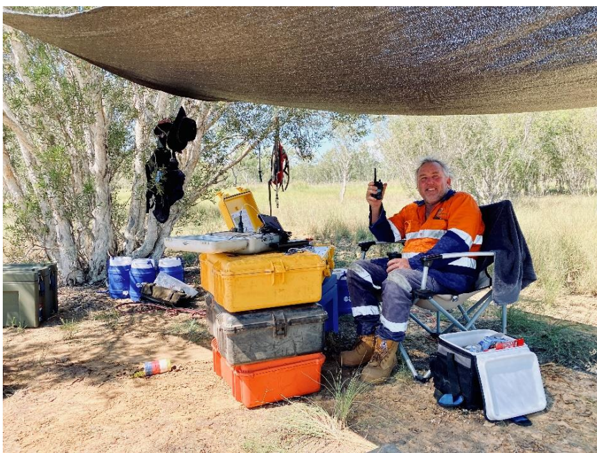
Figure 1: Image of the transmitter station as part of the FLEM survey at Orion, manned by Marty from the Southern Geoscience’s Niche Acquisitions team.
